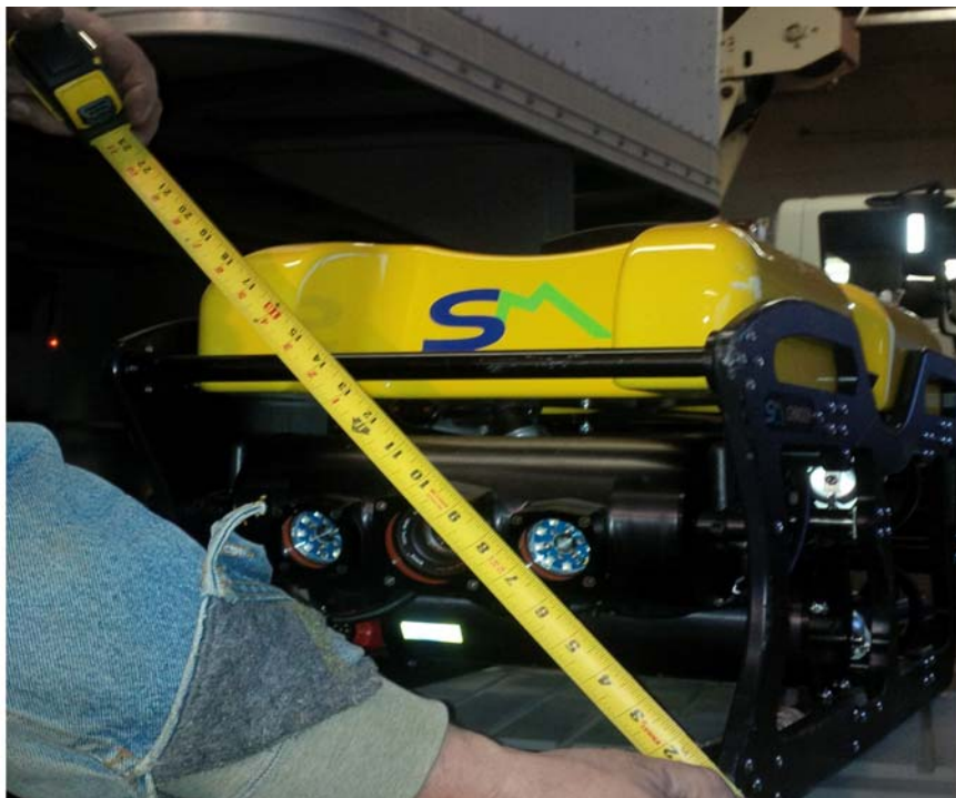
CCD Ltd Chinook ROV, will fit inside a 24" Pipe
